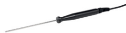
Hand-held temperature sensor, Figure 138 00 003 To measure water temperatures, in particular drink- ing water temperatures in the area of the outlet of the tapping points on site. Fast reacting sensor for detection of temperature fluctuations; temperature measurement range 0–150°C; 150 mm long meas- uring probe made of stainless steel; cable length 1.0 m.
